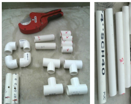
Materials needed to build the frame of the spat collector
