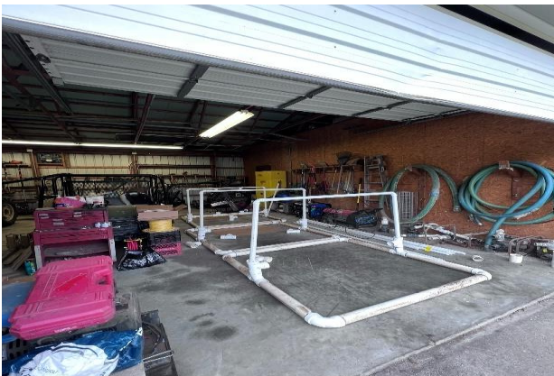
Assembly of frames of the rafts
