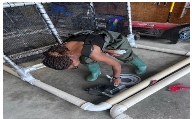
Attachment of water pump to raft
