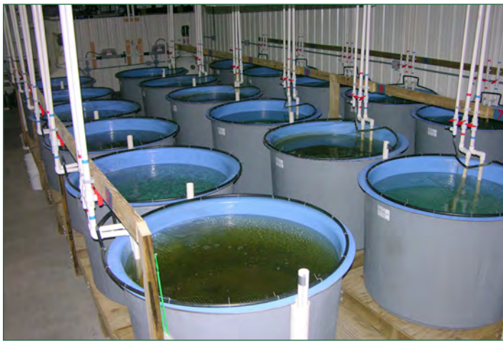
Here are two of the seven recirculating systems in the ARDF wetlab. Each of these tanks are 1000-L and can be randomly assigned to either of the systems in this array to optimize our experimental design. Photo: Lori Brown
